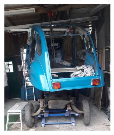
The scissor lift unit really makes life much easier on tasks such as these leaving the body dangling in the air.
